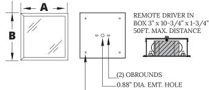
(4) 0.38" THRU HOLES for 2x2 (6) 0.38" THRU HOLES for 2x4
