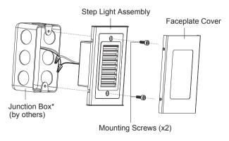
\*Outdoor rated junction box required for exterior applications.
