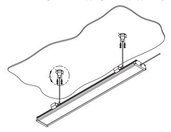
2. Suspend lamp with aircraft cable or stem (supplied by others) and then connect to the power.
