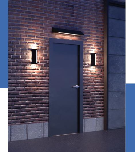
The Gateway Series offers field installation flexibility allowing light to be positioned right where you need it for the most effective egress lighting. With our patented adjustable locking mechanism, the optical chamber can be set in five different positions upon installation (-25°, -12.5°, 0°, 12.5°, 25°).
